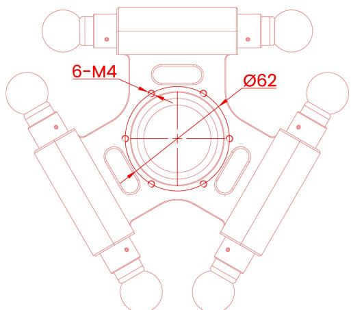
**基座安装 Base installation (mm)**
