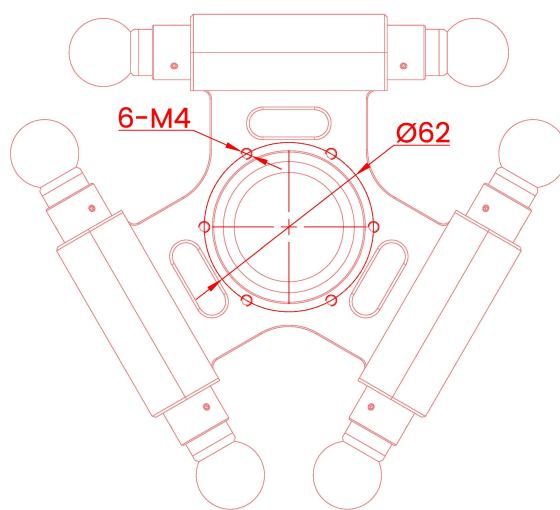
**基座安装 Base installation (mm)**
