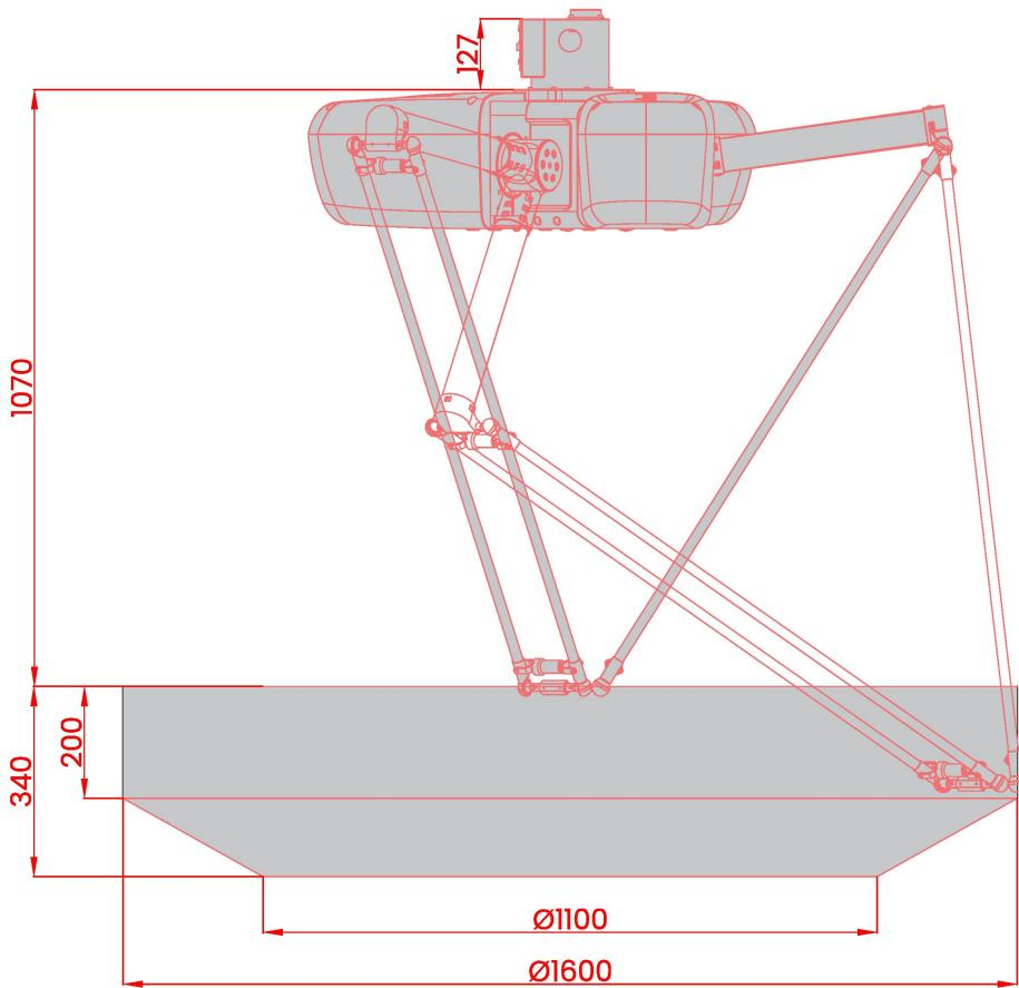
**法兰 Flange (mm)**
