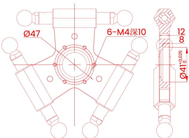
基座安装 Base installation (mm)
